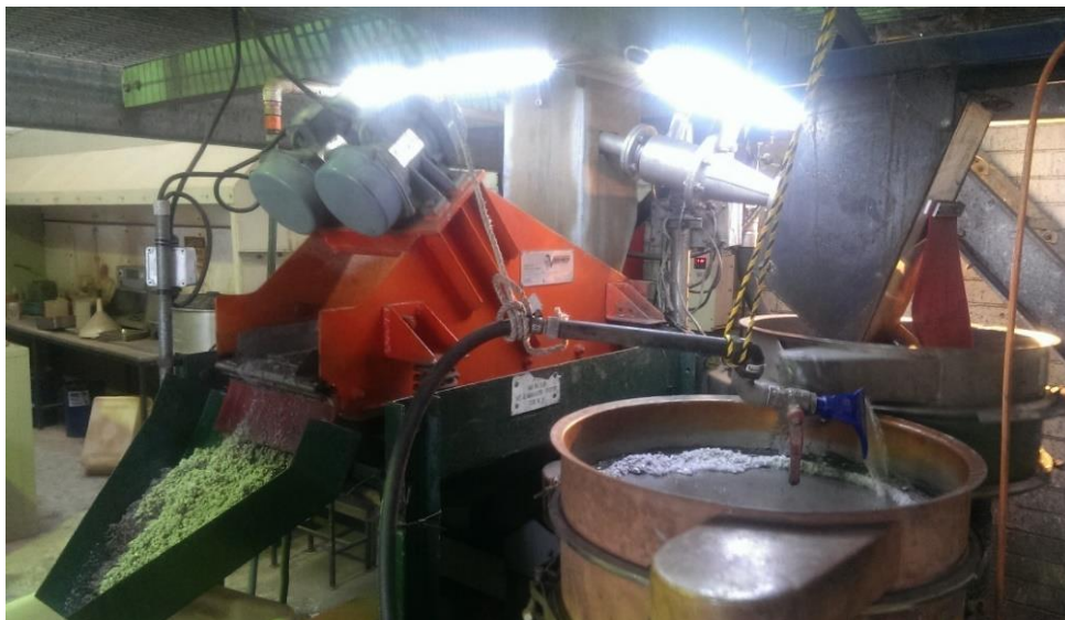
Figure 6: Left – HMS Spodumene-Tantalum Concentrate; Right – HMS Floats
