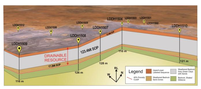
Figure 2: Schematic LD Cross-section Cut-out
