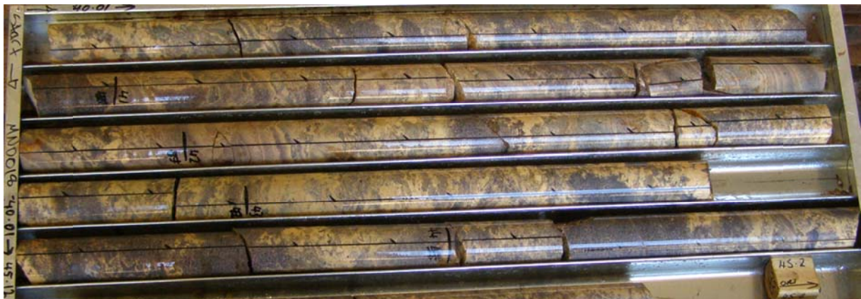
Figure 6: Diamond core from MND018 showing zone of purple coloured lepidolite. Assaying of this zone returned the highest assay result of 2.14% \text{Li}_2\text{O} from 43.36m to 44m. Photo shows diamond core from 40.01m to 45.12m.
