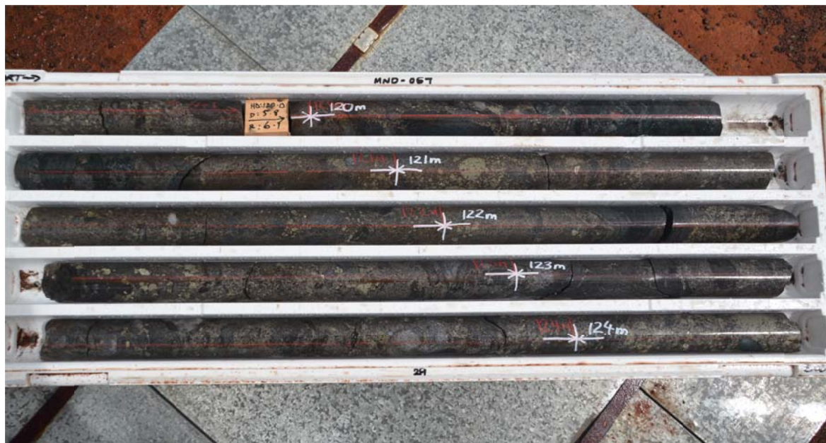
(Figure 3: Photograph showing drill core of the newly discovered 7.2 metre semi-massive sulphide zone within the felsic rock sequence below the existing defined resources at Kultarr.)
