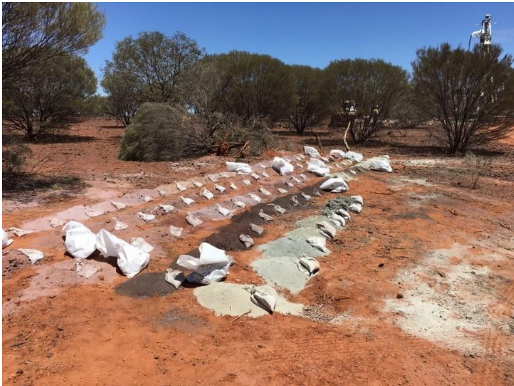
Figure1: Samples from the Company's Maiden RC Drilling Program completed over the Project in March 2017 – dark brown piles are massive magnetite zone
