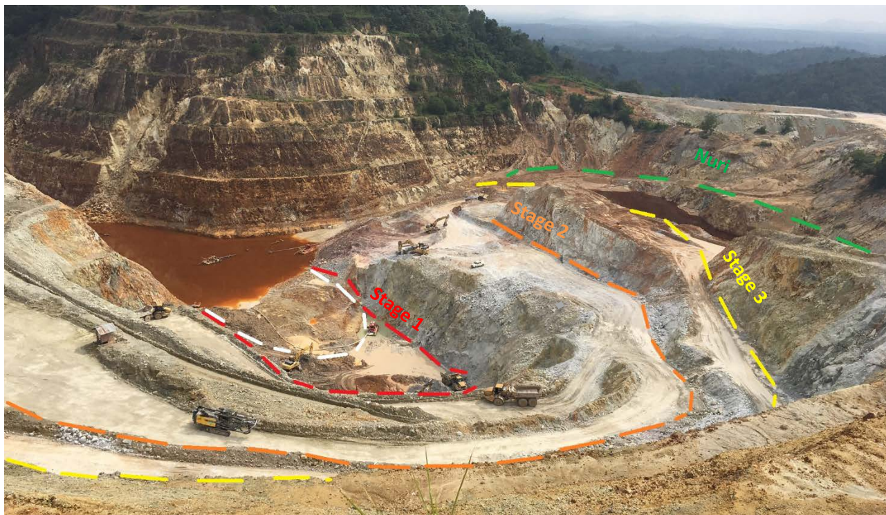
Figure 5. Berenai pit showing mud removal. The white dashed line depicts the additional mud area which was in the mine plan as stage 1 ore and has now been shown to have been historically mined.
