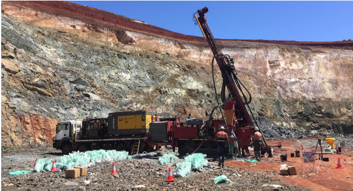
RC Drill Rig In Progress within the existing Orelia Open-pit
