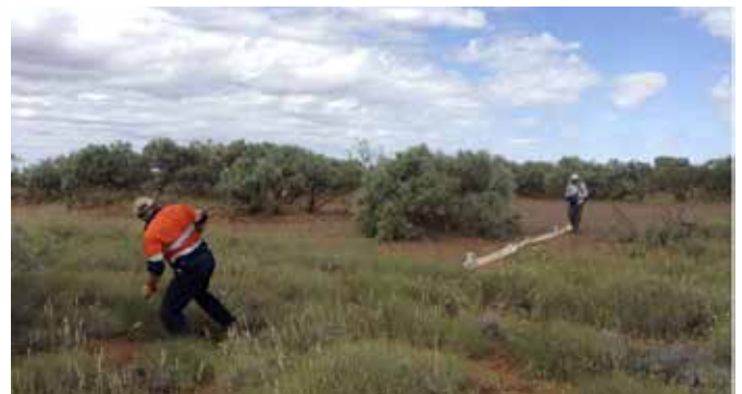
Figure 10 – Manual towing of the DGPR sensor array during the trial survey at Manyingee East.
