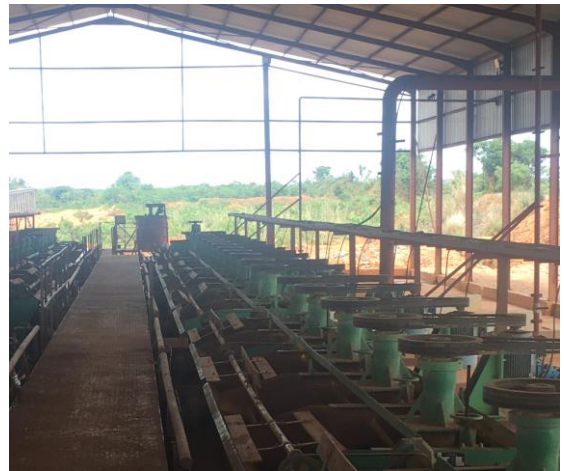
Kipushi Processing Plant - Flotation Cells and Ball Mill
