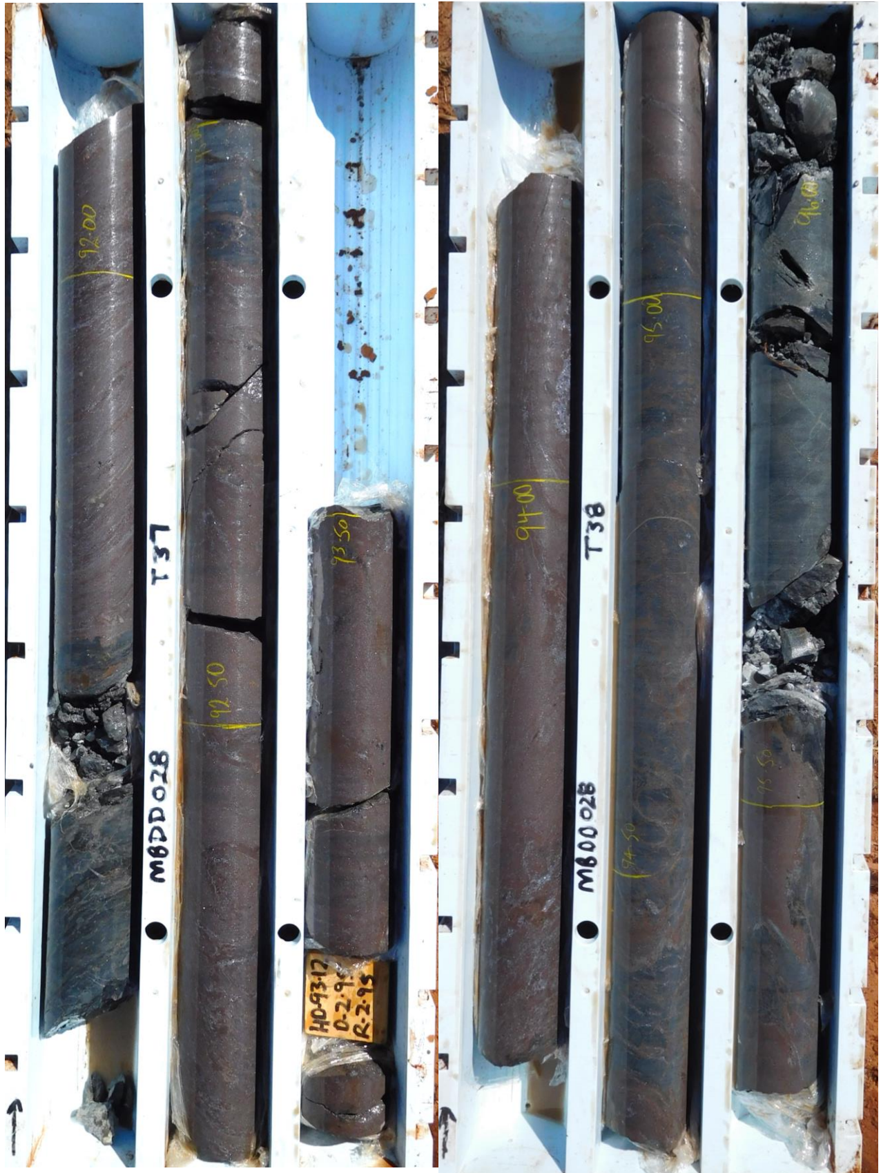
Figure 1 – MBDD028 sphalerite-galena dominant massive/semi-massive sulphide (91.5-95.5m)
