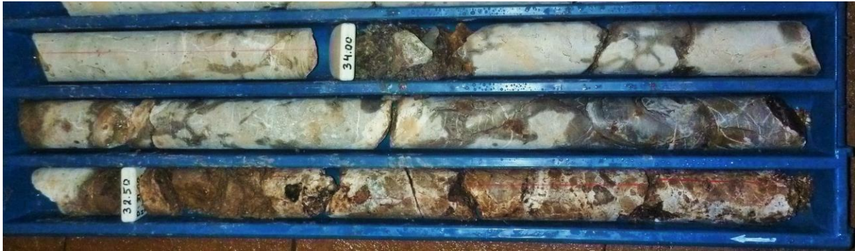
Figure 10: ABOVE Core tray photo of RDDH-001 near to its current depth (at the time of writing). The core shows strong brecciated and development of gossan horizons (weathered sulphides).
