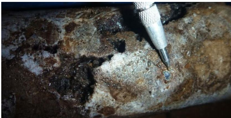
Figure 9: LEFT Core photo RDDH-001 (Humaspunco) showing gossan (weathered sulphides) and fresh sulphide (galena blebs) in a brecciated limestone.
