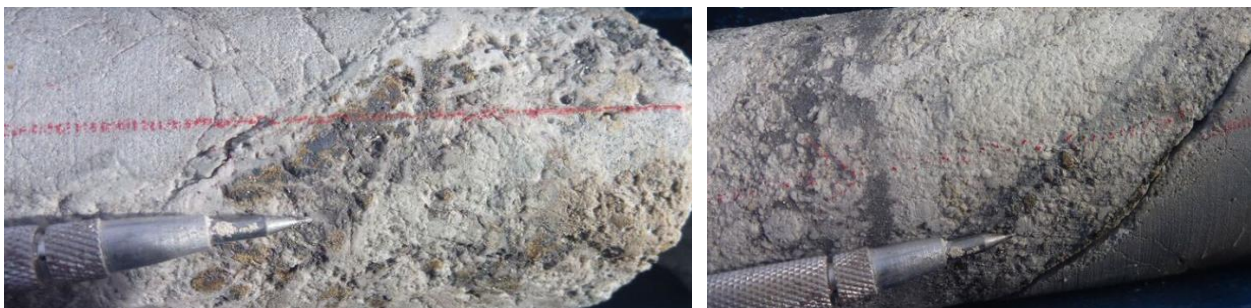
Figure 7: ABOVE RDDH-009 core photos from fourth mineralised structure zone; strong sulphide development as zoned disseminations or open veins comprising pyrite, galena, sphalerite and chalcopyrite within argillic altered volcaniclastics.
