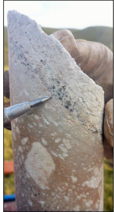
Figure 3: RIGHT Highly altered porous volcaniclastic rock (between 137.1m to 137.4m) with veinlets of sphalerite, galena and chalcopyrite in RDDH-009 (Uchpanga).
