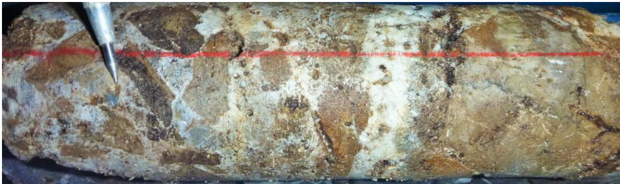
Figure 11: ABOVE Core photo of upper parts of RDDH-001 (Humaspunco) showing a mineralised brecciated manto or vein. Several clasts are gossanous (dark red-brown). Coarse galena blebs occur in the matrix of the breccia.
