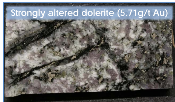
Strongly altered dolerite (5.71g/t Au) Quartz-biotite-albite-sulphide altered quartz dolerite (cf. Junction gold deposit, St Ives)
