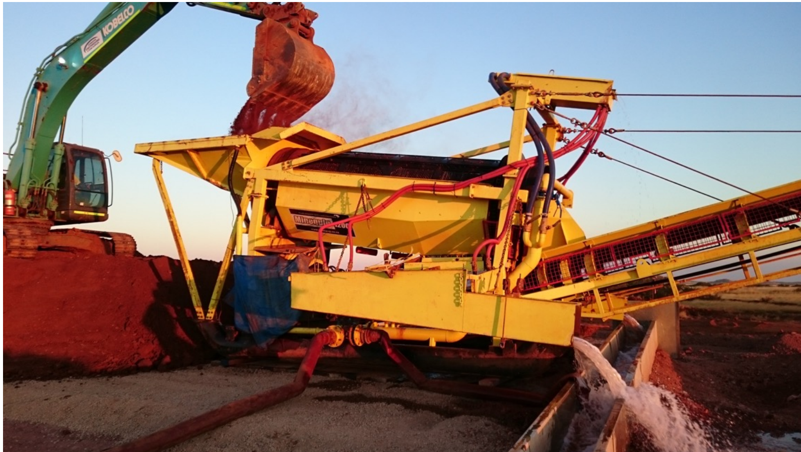
Mobile 1200-XT Gravity Gold Plant at Nickol River for bulk sample testwork
