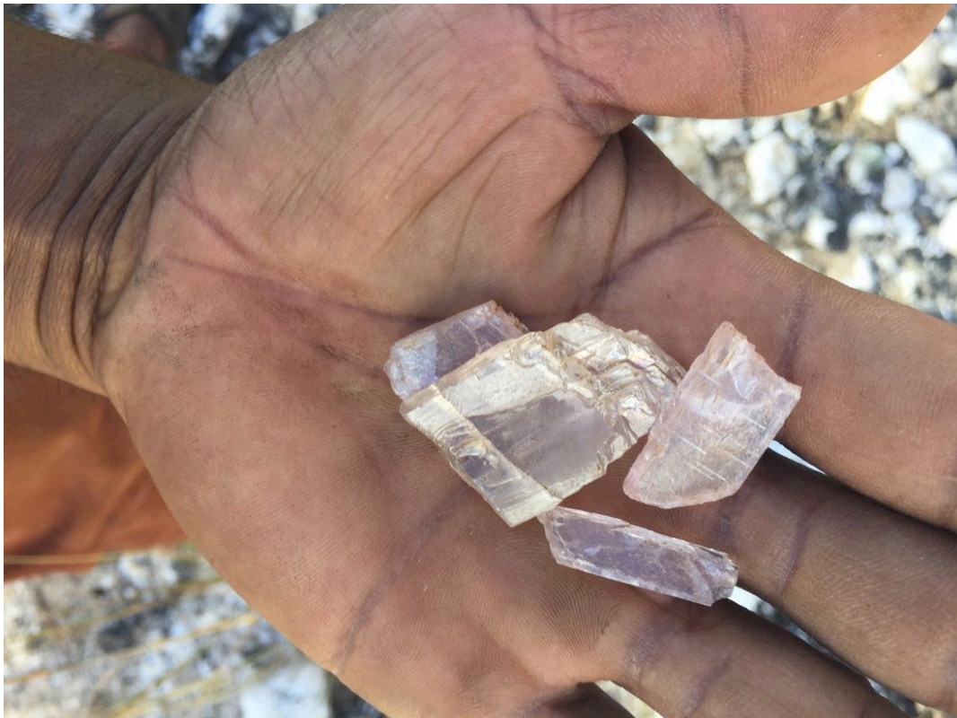
Figure 1: Samples of high purity Spodumene crystals (Kunzite) found in the project area.
