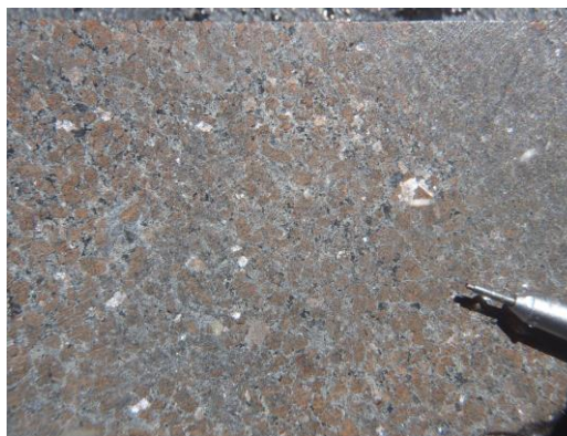
Figure 2b. Hole LV5016 96.8m; Granular crystals of sphalerite and minor pyrite showing similar textures to mineralisation intersected in TRSDD010
