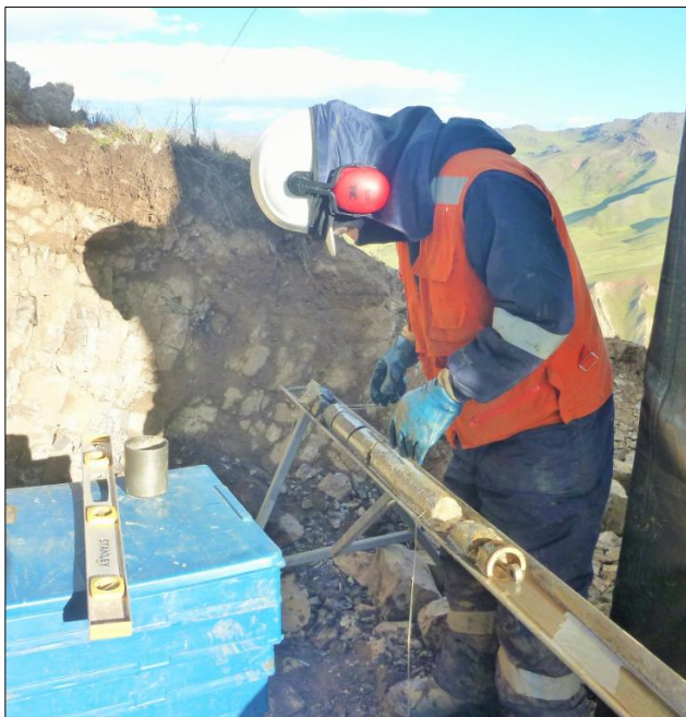
Figure 2: LEFT Taking core orientation measurements at RDDH-001.
