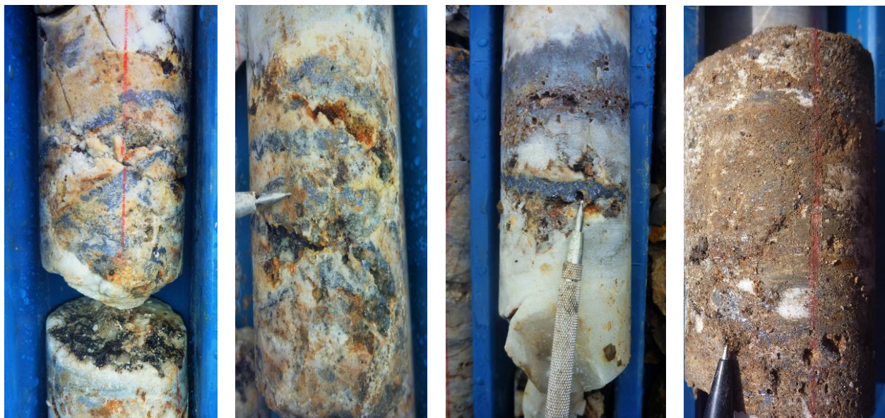
Figure 1: ABOVE Core photos of RDDH-001 (Humaspunco) showing mineralised zones most likely associated with Zn-Ag-Pb veins HV-09 and HV-06. LEFT THREE Smithsonite (a rich Zn-bearing carbonate) and galena (lead sulphide) in HV-09 FAR RIGHT Semi-gossanous (oxidised sulphides) and streaks of fresh galena in HV-06. Refer also to Figure 4.
