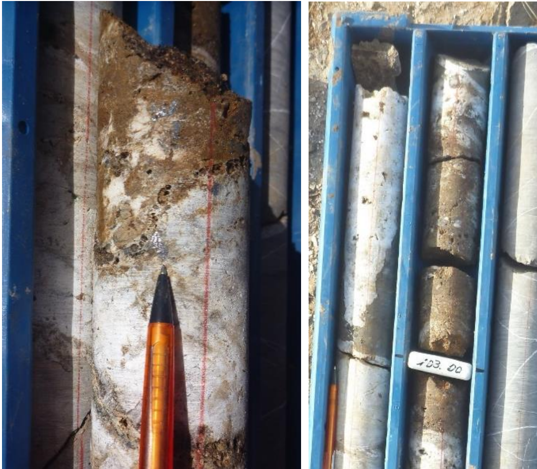
Figure 4: ABOVE Additional core photos of the mineralised zone associated with HV-06. Coarse blebby galena is highlighted.
