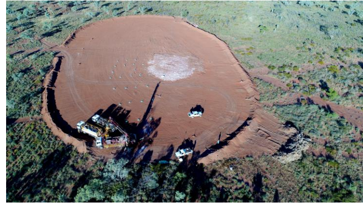
Gambit West – topsoil cleared and grade control drilling commenced
