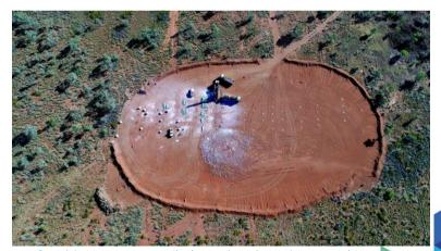
Gambit West - topsoil cleared and grade control drilling commenced
