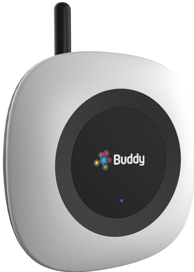
Figure 1. Introducing Buddy Ohm Link – extending the size and sensor volume of Ohm systems
