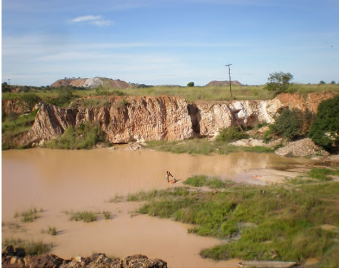
Carrier de l'est pit Manono Zone. Showing pegmatite dipping quite flat at around 17 degrees SW
