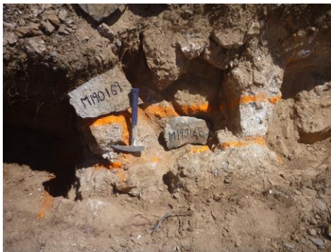
Figure 2: ABOVE HV-10 in outcrop - photo showing one of the channel sample sites; MIDDLE HV-10 rock specimen showing gossanous sulphides with visible galena (silver-grey); RIGHT HV-10 in drill core showing partially weathered sulphides (Fe-coated galena - brown) and visible malachite (green).
