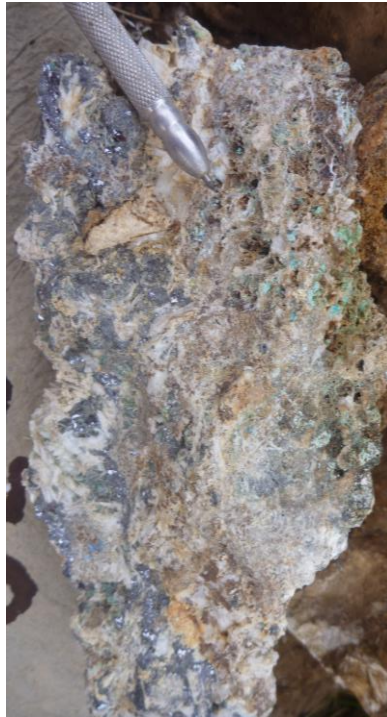
Figure 4: ABOVE HV-06 in outcrop - photo showing one of the channel sample sites; MIDDLE HV-06 rock specimen showing partially weathered sulphides with visible galena. Smithsonite and secondary copper are also present; RIGHT HV-06 in drill core showing highly weathered sulphides (Fe-coated galena - brown) with relict fresh galena visible (silver-grey patches).
