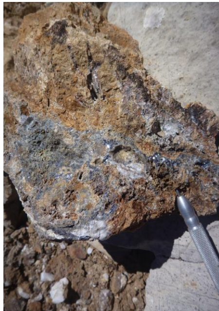
Figure 2: ABOVE HV-10 in outcrop - photo showing one of the channel sample sites; MIDDLE HV-10 rock specimen showing gossanous sulphides with visible galena (silver-grey); RIGHT HV-10 in drill core showing partially weathered sulphides (Fe-coated galena - brown) and visible malachite (green).
