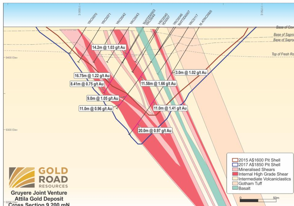
**Figure 5:** Section 9,200 mN illustrating the internal high-grade zones that have been delineated and the interaction between the Footwall and Main shears, developing broad zones of mineralisation. Showing the 2015 and 2017 optimised pit shell outlines
