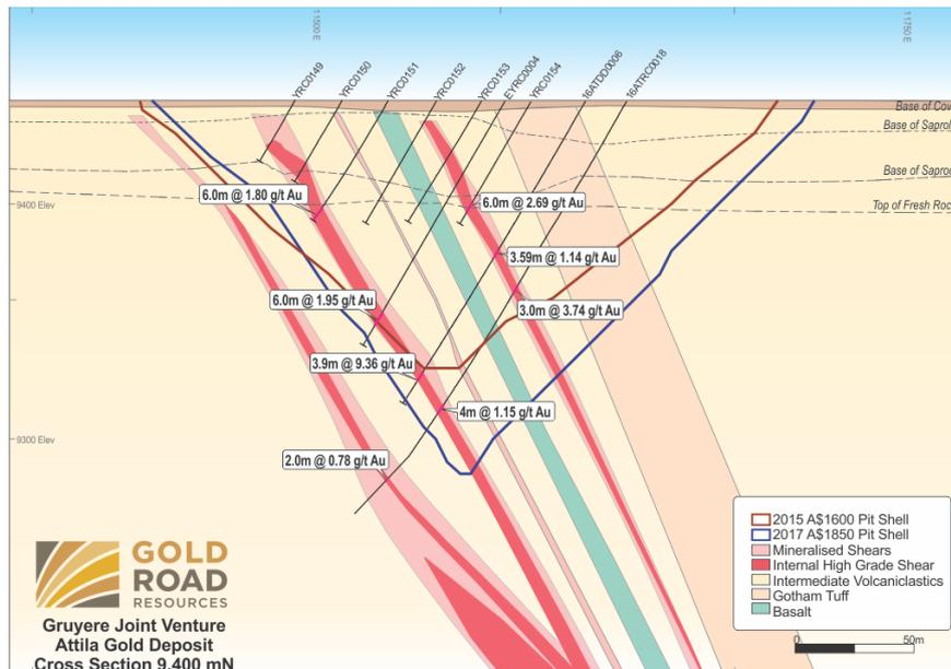
**Figure 6:** Section 9,400 mN illustrating the internal high-grade zones that have been delineated and the interaction between the Footwall and Main shears, developing broad zones of mineralisation. Showing the 2015 and 2017 optimised pit shell outlines
