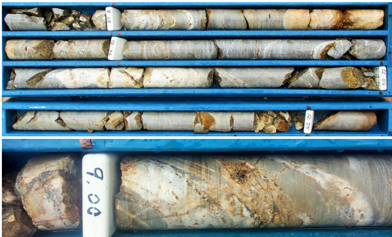
Figure 1: ABOVE TOP Core tray photo of the new mineralised structure intersected at 8.9m down hole depth. ABOVE BOTTOM Detail at 9.0m depth showing relict sulphide (mainly galena) veinlets that parallel and cut across an earlier set of sulphide-bearing calcite-barite veins, which contain trails of disseminated galena and pyrite.
