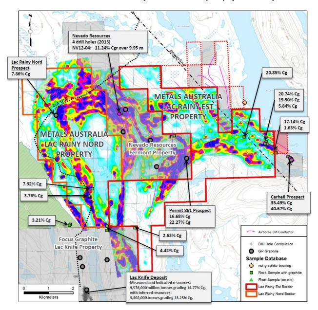
Figure 1: Results of the MAG and TDEM Surveys – Lac Rainy Nord and Lac Rainy Est Graphite Projects, Quebec,
