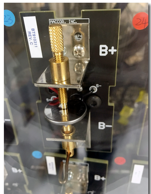
Figure 1 Talga GNP Li-ion battery being tested in climate cabinet rack.
