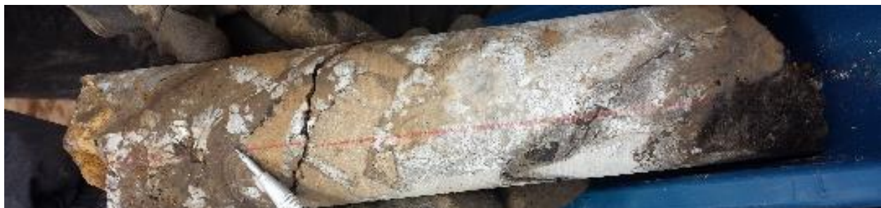
Figure 3: ABOVE Core photo at 115.8m in RDDH-004. An example of mineralisation at modest depths in drilling at Humaspunco. Fe-oxides (red-brown) and cream-coloured minerals which mostly comprise the gangue minerals (calcite and barite).
