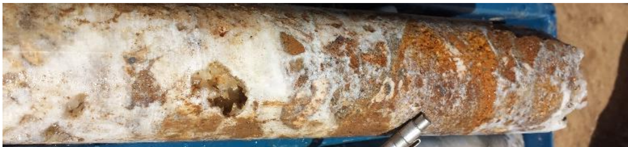
Figure 2: ABOVE Core photo at 90.5m in RDDH-004. This is typical of mineralisation at shallow depths in drilling at Humaspunco. Relict galena (grey-silver) with Fe-oxides (red-brown) and calcite and barite (cream-coloured), which mostly comprise the gangue minerals.
