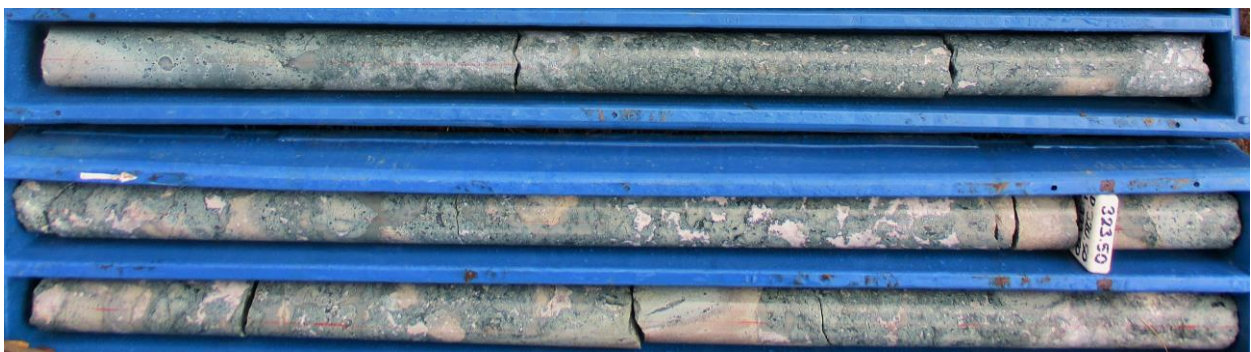
Figure 4: ABOVE Core tray photo of the sub-volcanic. It is strongly chloritized (green colouring) and hosts disseminated pyrite. It is a complex rock with multiple zones of brecciation, intervals of intense “eyes” (concretions and/or volatile infillings), alteration and veining.
