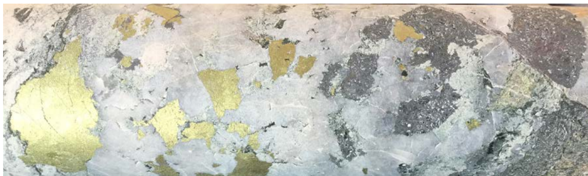
Quartz-calcite veining with chalcopyrite-magnetite-hematite associated with a mineralised zone in HDD001 (307m)
