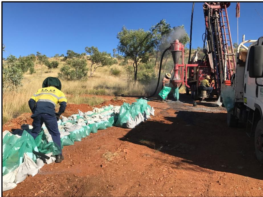
Figure 4 – Drilling rig in operation at Burke Graphite Project
