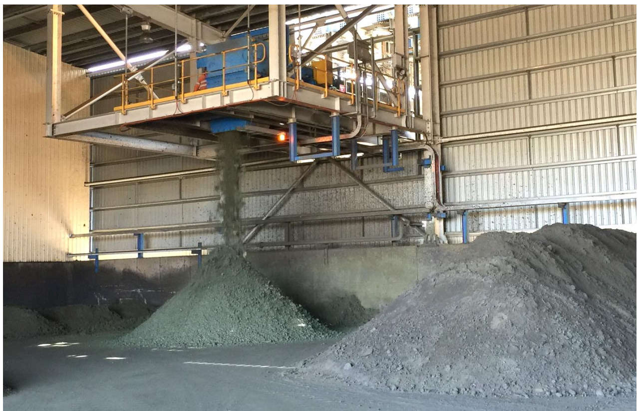
Figure 02: June concentrate (under the chute) is some of the best to date. Remaining May concentrate yet to be shipped (right) was impacted by low recoveries and lower concentrate grades due to blending of ore types with conflicting processing methodologies.
