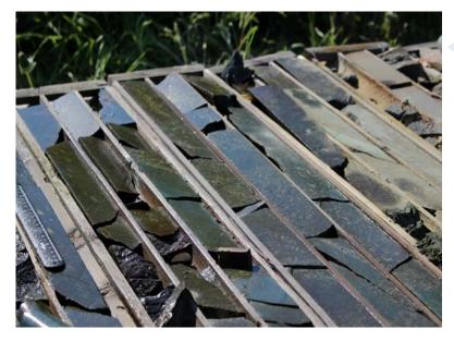
Extensive zones of gabbrohosted, massive to disseminated sulphide mineralisation, including pyrite, chalcopyrite, and pentlandite, was seen in the core (see adjacent photo).
