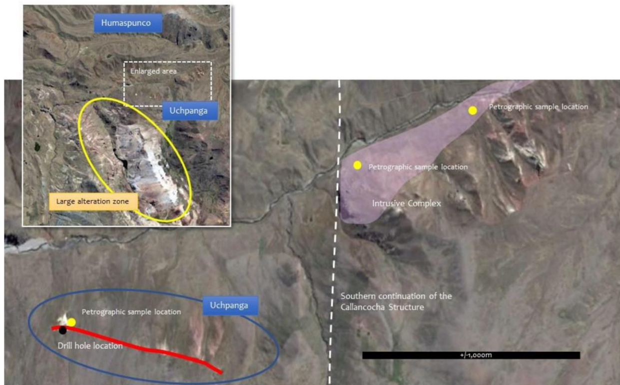
Figure 4: ABOVE Satellite image of the southern third of the Riqueza project area. The drilling at Uchpanga (black dots – refer also to Figure 2, is shown relative to the 750m long gossan (red line). The intrusion east of Uchpanga is shown as well as the large alteration zone that is south of Uchpanga (insert image).
