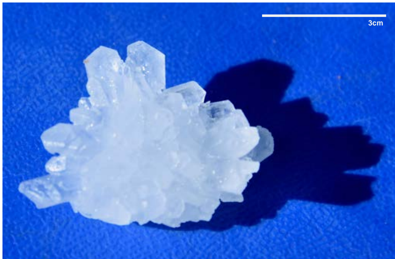
Figure 7: Sample of Kainite Salt Crystals from Lake Wells Site Evaporation Trial
