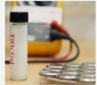
The graphite is replaced by titanate powder.
