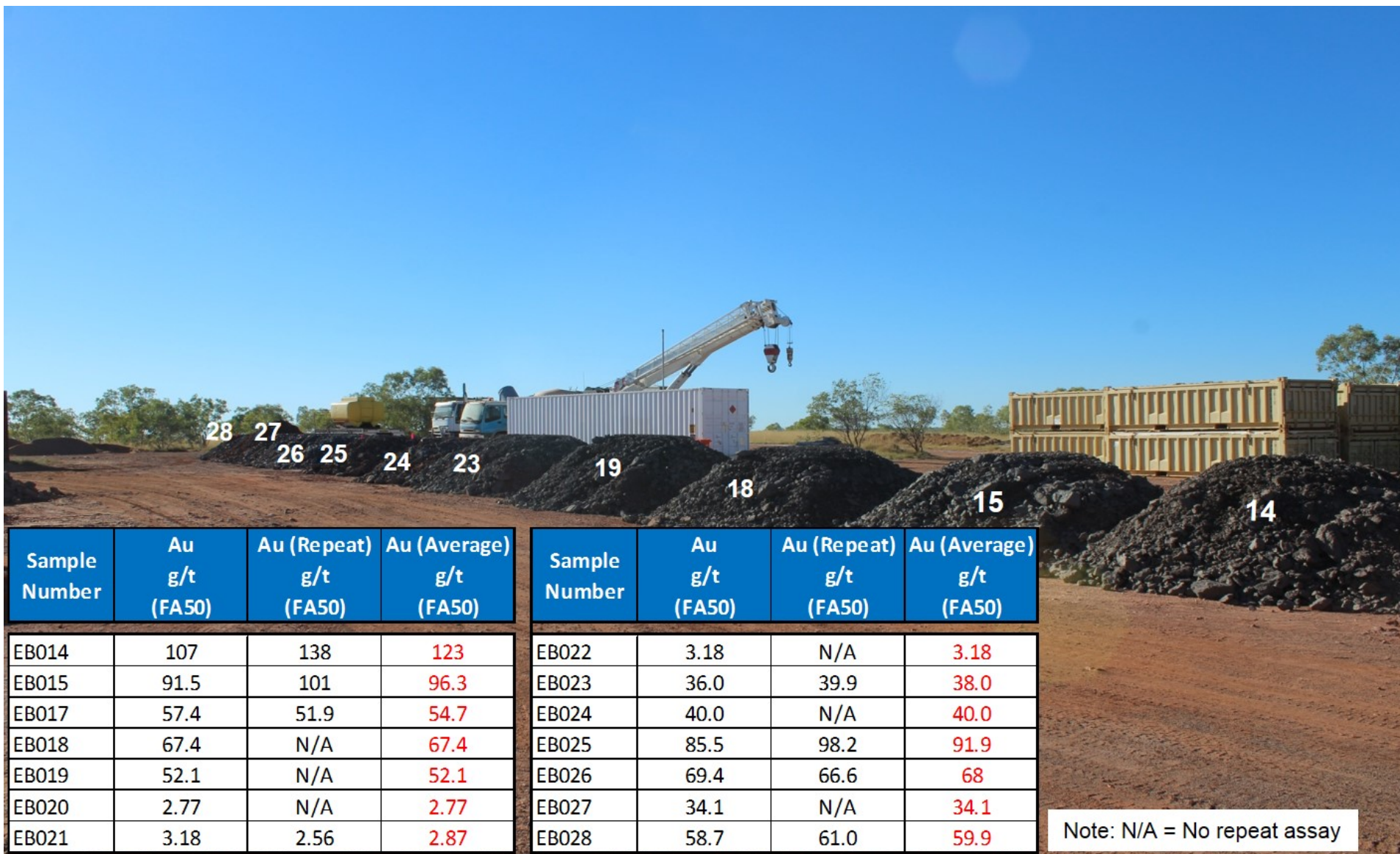
Figure 4: Development Ore on the ROM Pad at the Edna Beryl Mine. Note the gold assay results from the bulk samples
