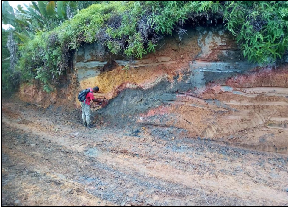
Graphite seam with adjacent disseminated zones exposed in road cut in Main Zone
