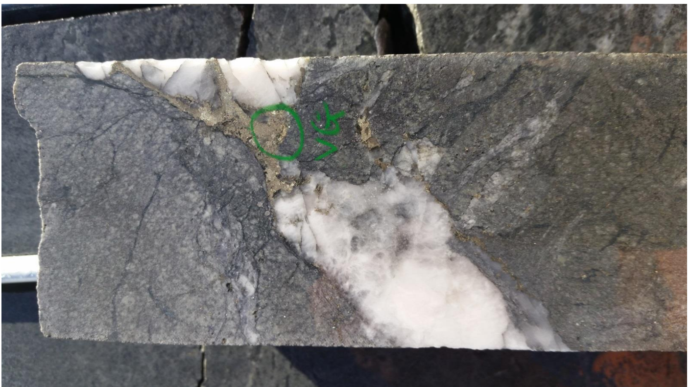
Figure 7: Photograph of ½ drill core BORCD 179 (348-349m) visible gold assayed 1.69 g/t Au,
