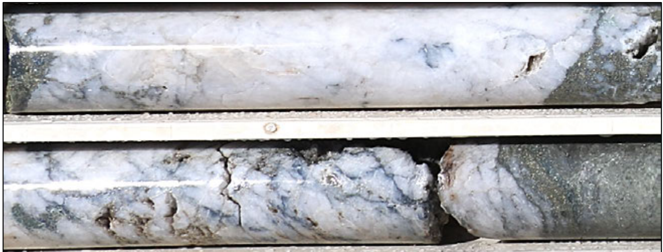
Figure 2 - AWT002 drill core at 211.5 metres (top row) and 212.5 metres (bottom row). Stringer molybdenite in massive quartz vein with intense sericite altered and pyritic wallrock. Host unit is a clay altered, chlorite-actinolite greywacke.
