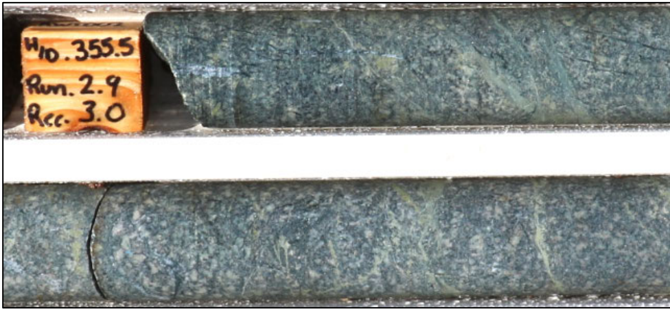
Figure 8 - AWT002 at 355.5 and 356.5 metres. Coarsely crystalline quartz- feldspar-phyric quartz monzonite porphyry with strong selective actinolite-epidote-chlorite alteration and stringer quartz-epidote-clay veins and fracture fill.
