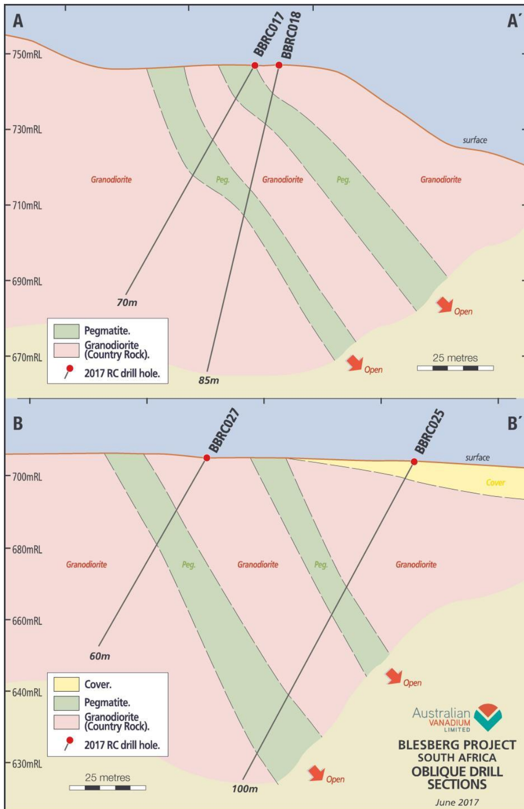
Figure 2a. Geological Section – Blesberg Historical workings looking SE Figure 2b. Geological Section – P1 Area, NW extension of Blesberg looking SE
