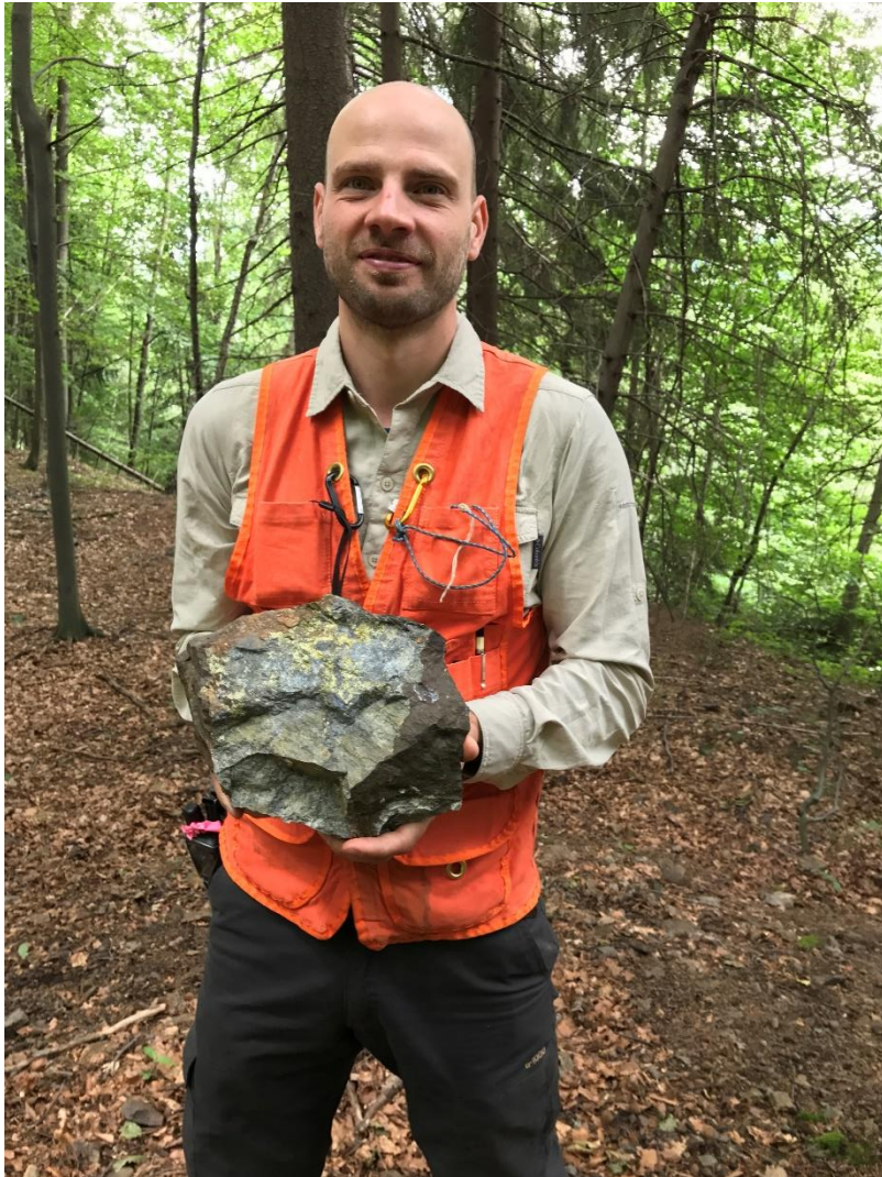
Figure 3: Chief Geologist, Sven Honig holding a sample of mineralisation from Pavol Waste Dump with stringer and disseminated copper and cobalt sulphides
