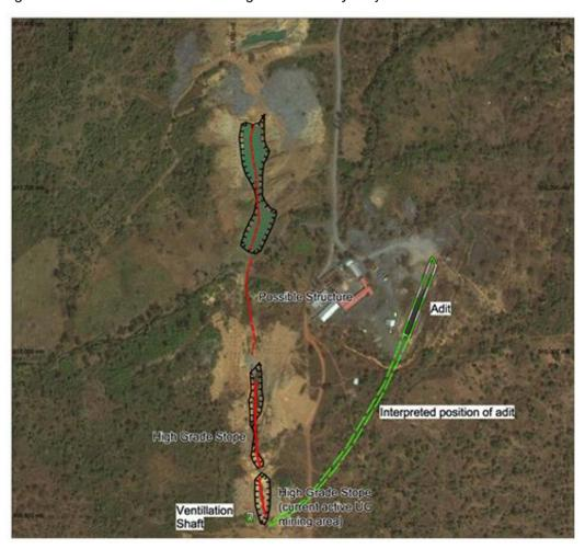
At the Tawny Project, Zn/Pb (Ag) mineralisation is found within an easterly dipping fault zone. The north/south trending fault structures hosting the mineralisation have excellent strike continuity with expected pinch and swell boudinaged higher-grade zones present.
