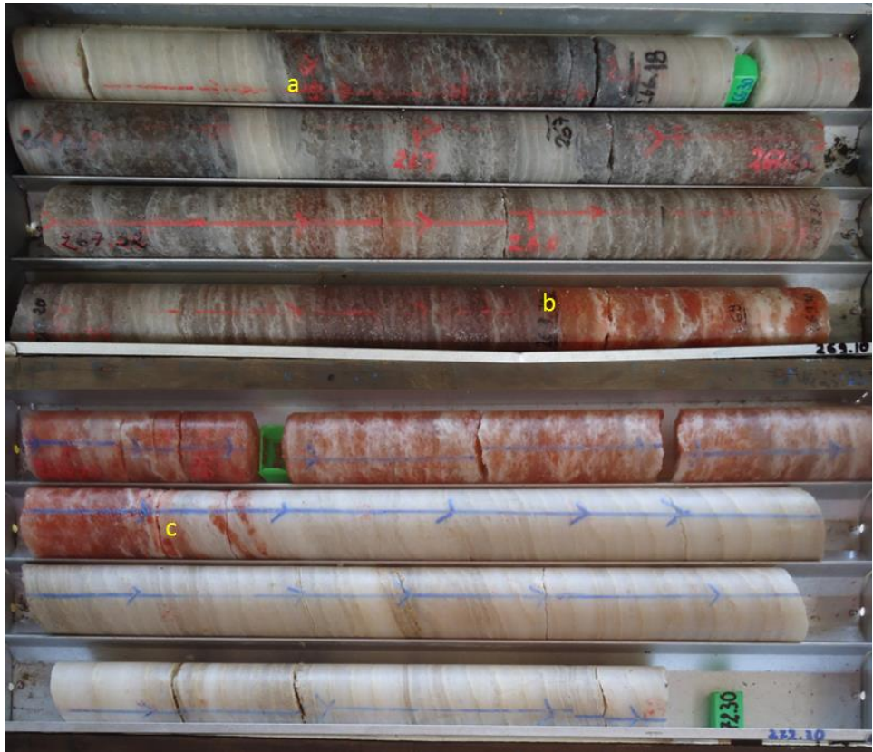
Figure 16. Photograph of (PQ size) core from an intersection of Upper Seam in drill-hole EK_38. The seam is partially replaced; the upper part of the seam (a to b) is Sylvinite (USS) and the lower part (between b and c) is Carnallitite (USC). Classified as 'type B' seam (as per Table 4 below). The easily identifiable and abrupt nature of the contacts is visible.
