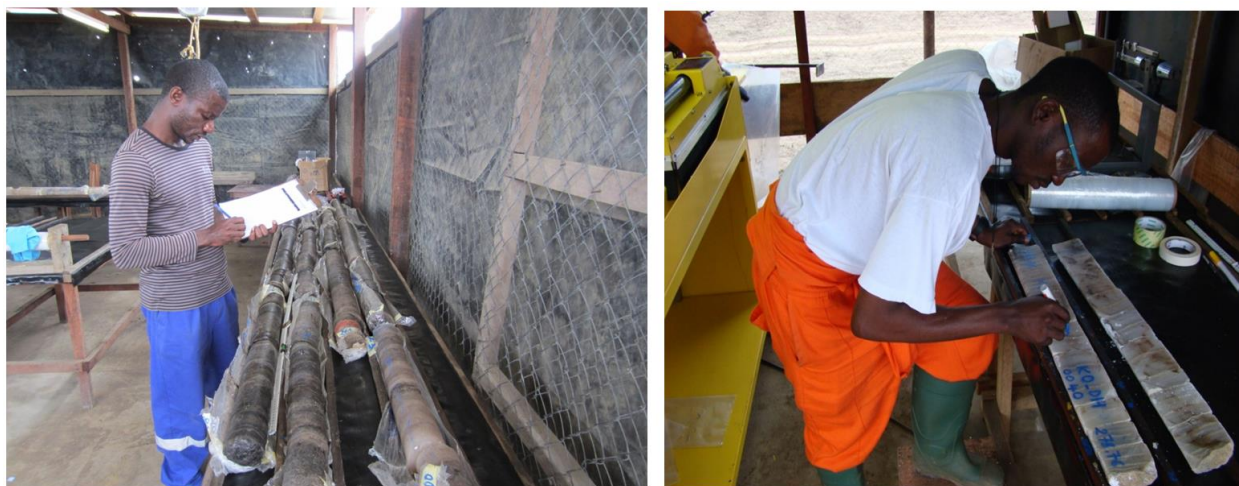
Figure 2 Left: logging the core. Right: Labelling the cut core, one half for analysis the other retained as a record
