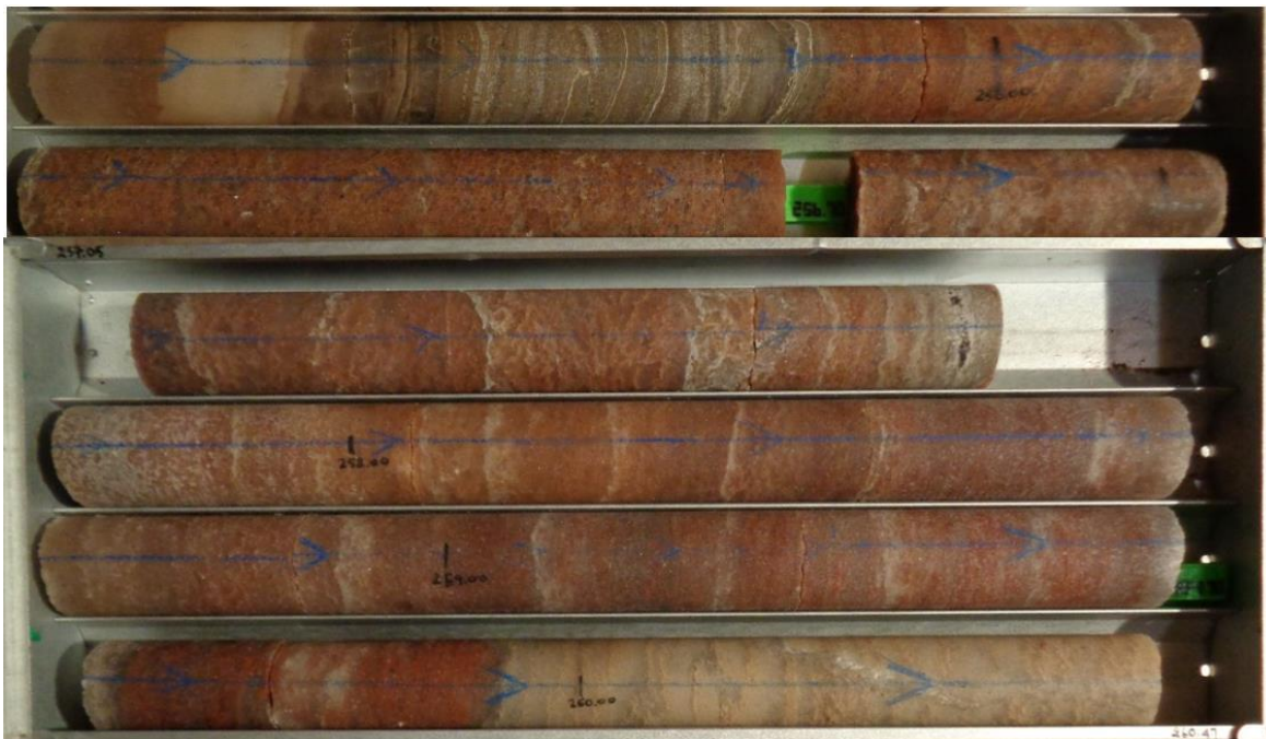
Figure 1 Whole PQ sized core shortly after drilling, Sylvinitic clearly visible as the orange-red rock type. The seam in this example is the Hangingwall Seam Sylvinitic comprised between 50 and 60% sylvite . The easily identifiable and abrupt nature of the contacts is visible.
