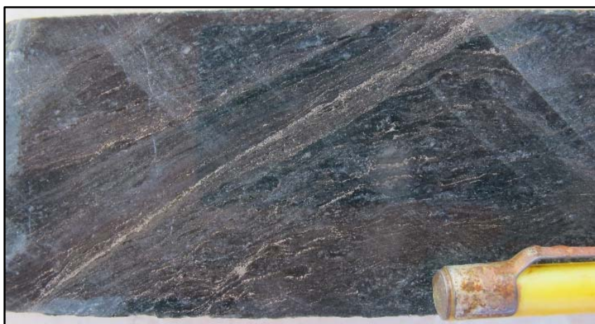
BBDD0010: 5.3m @ 7.07g/t gold from 244m (laminated, sulphide-rich lode; ASX Release 30 May 2017)
