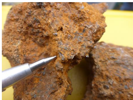
Figure 5: ABOVE LEFT Wall rock photo inside the Vilcapuquio mine working (upper level) showing a broad zone of highly altered stockwork veining (brown discolouration). ABOVE RIGHT Photo of a rock sample taken from this section of the mine. The sample grades 42.77% Zn, 3.4g/t Ag and 2.73% Pb.
