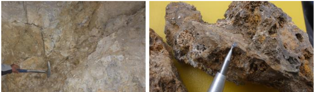
Figure 5: ABOVE LEFT Wall rock photo inside the Vilcapuquio mine working (upper level) showing a broad zone of highly altered stockwork veining (brown discolouration). ABOVE RIGHT Photo of a rock sample taken from this section of the mine. The sample grades 42.77% Zn, 3.4g/t Ag and 2.73% Pb.
