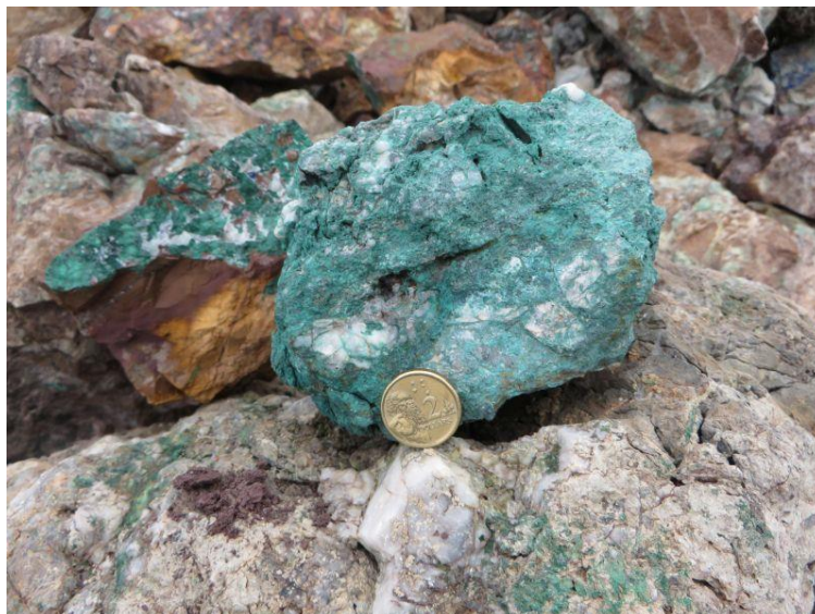
Figure 7: High grade copper (malachite) mineralisation, Thaduna Mine
