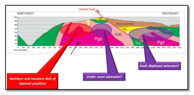
Figure 3– Schematic section showing the exposed porphyry system which has been drill tested, its likely covered extension to the East, and the low angle Chololo Fault that has potentially offset the upper part of the porphyry system, possibly preserving the typically higher grade phyllic alteration zone in the hanging wall of the fault under cover further to the South East.
