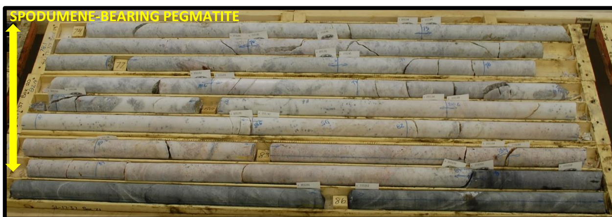
Figure 1. Drill core obtained from drill hole SL-17-37 showing the intersection of high-quality spodumene-bearing pegmatite (the lighter coloured material in the photo is the Pegmatite, whilst the darker material is Mafic Volcanic).
