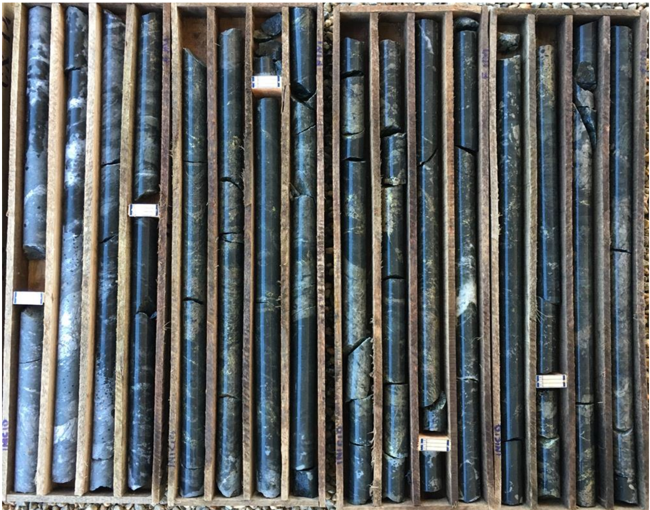
Figure 1: AAND-114 Upper Part of Mineralisation, Chalcopyrite and Gangue Sulphides
