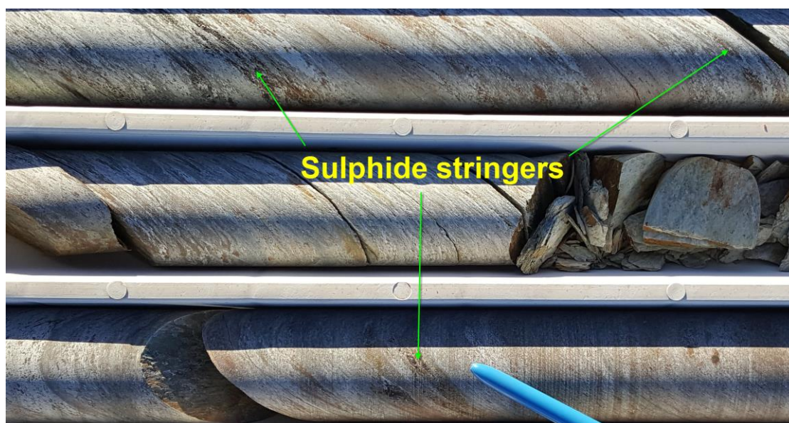
Figure 5: Existing diamond drill core with uncut disseminated (stringer?) base metal mineralisation from the Conquistador Prospect
