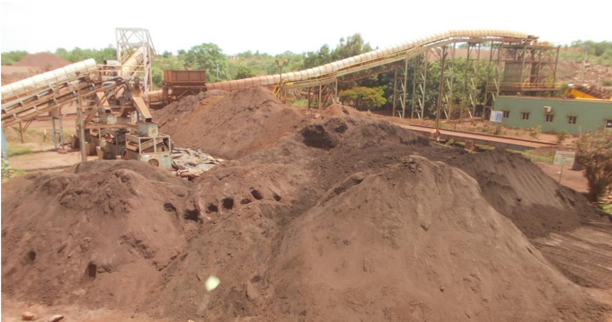
60/61% Fe stockpile and 62/63% Fe stockpile
