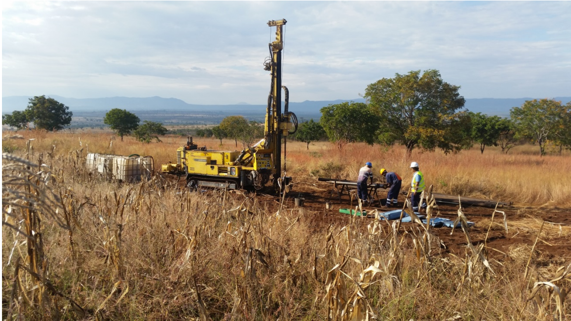
Figure 1 – Diamond Drill Rig on site at Longonjo, May 2017
