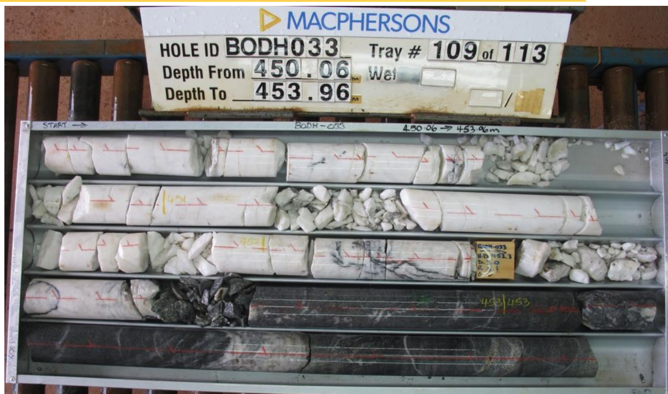
Figure 6: Diamond Drill Core BODH 033 – Laminated Quartz Vein with visible gold 452-453m (10.25 g/t Au)
